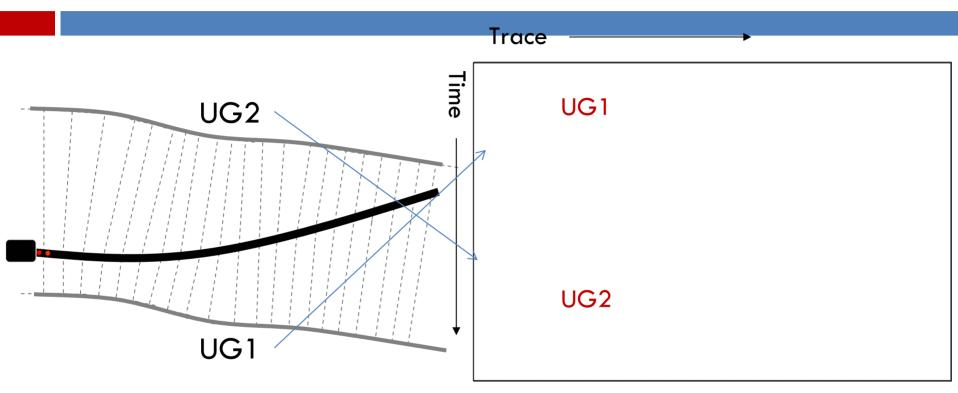
Borehole radar is non-directional. This means that we cannot tell which direction a reflection has come from. However GeoMole have developed procedures to overcome this. These procedures include but are not limited to forward modeling techniques that take into consideration the curvature of the drillhole or the use of multiple neighboring drillholes.
