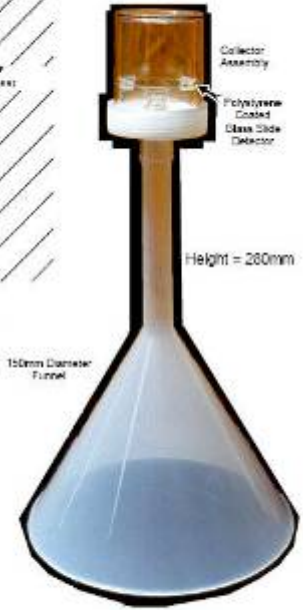
pSirogas Collector Design and Deployment Arrangement (Mark 3 or "C2" version of Detector)
