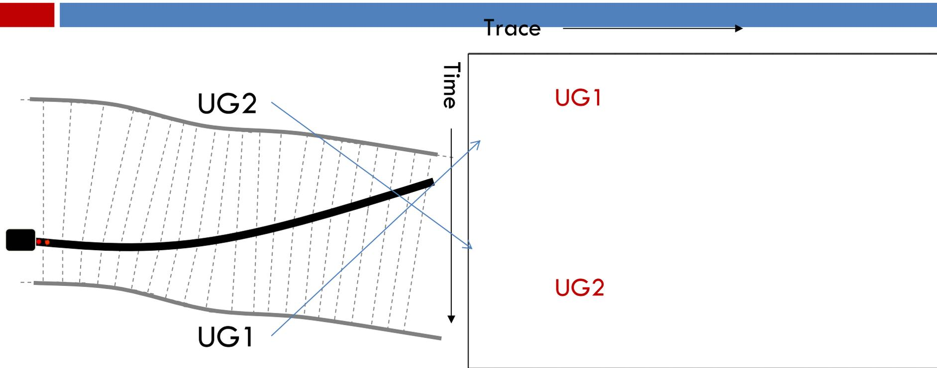
Borehole radar is non-directional. This means that we cannot tell which direction a reflection has come from. However GeoMole have developed procedures to overcome this. These procedures include but are not limited to forward modeling techniques that take into consideration the curvature of the drillhole or the use of multiple neighboring drillholes.
