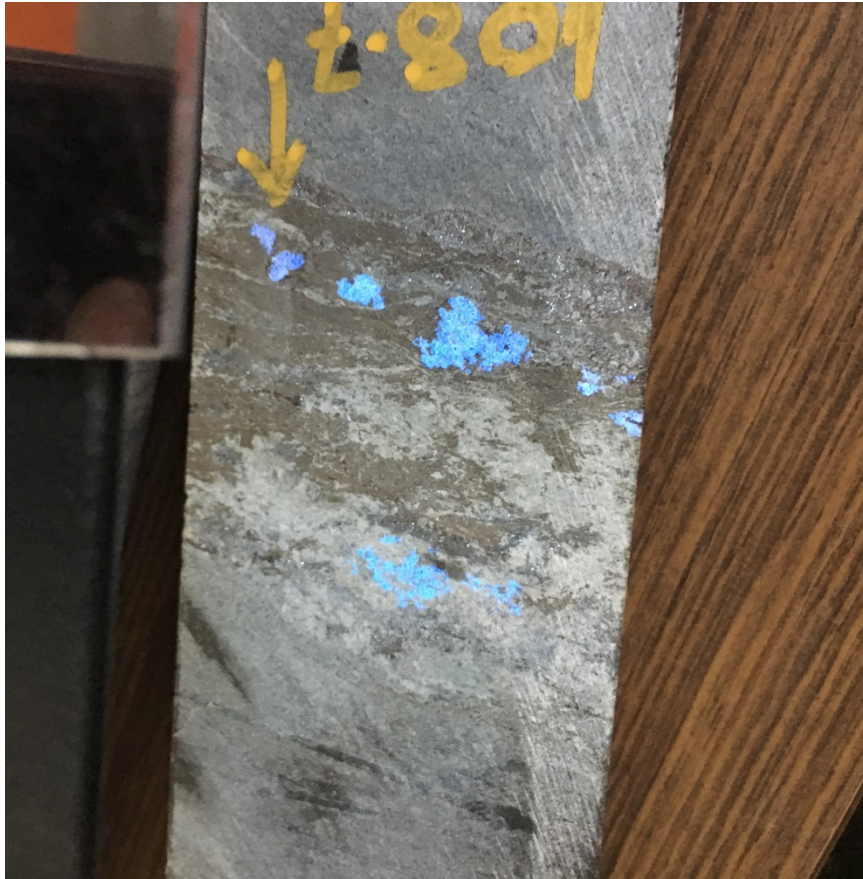
Sphalerite-galena-tremolite-garnet veins with abundant scheelite (under shortwave UV light), Far West Lower
