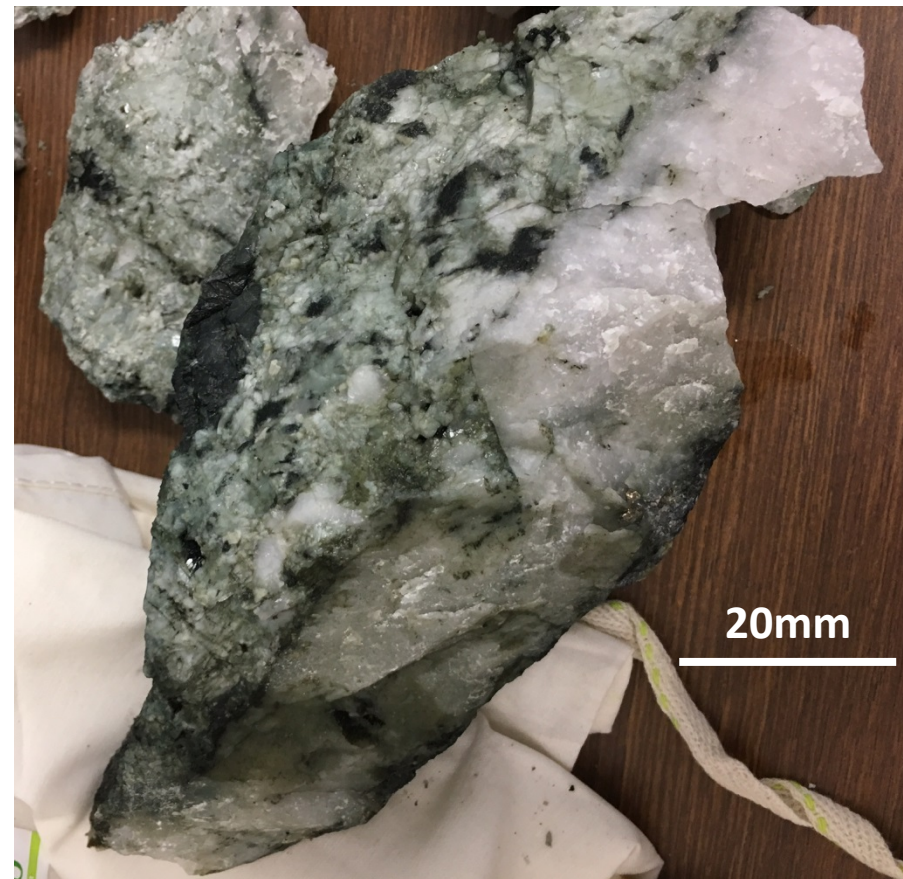
Massive albite (pale green) and quartz veining, 285SR Drive, Main South Lode. Dark patches are Fe-Chlorite
