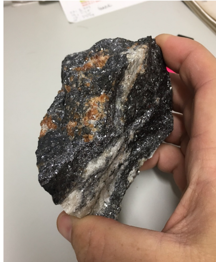
Recrystallised calcite, garnet, high-iron sphalerite and galena, 360SA Stope
