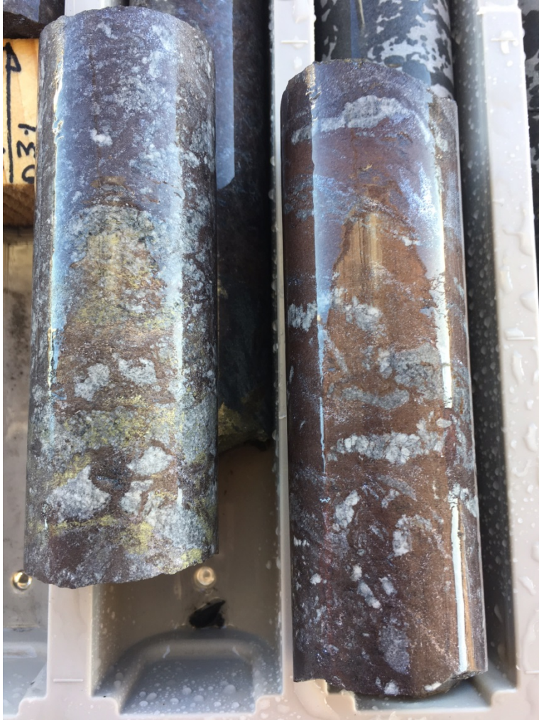
Dolomitic carbonate clasts in massive sulphide breccia
