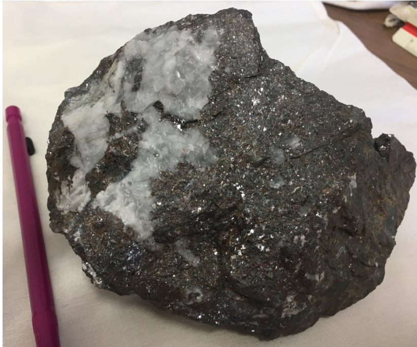
Calcite clasts (with minor tremolite) in sulphide breccia, 535FWS Drive, Far West Lode
