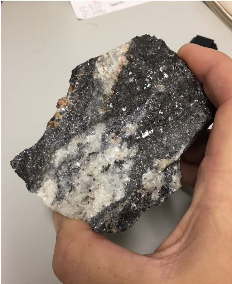
Recrystallised calcite, garnet, high-iron sphalerite and galena, 360SA Stope
