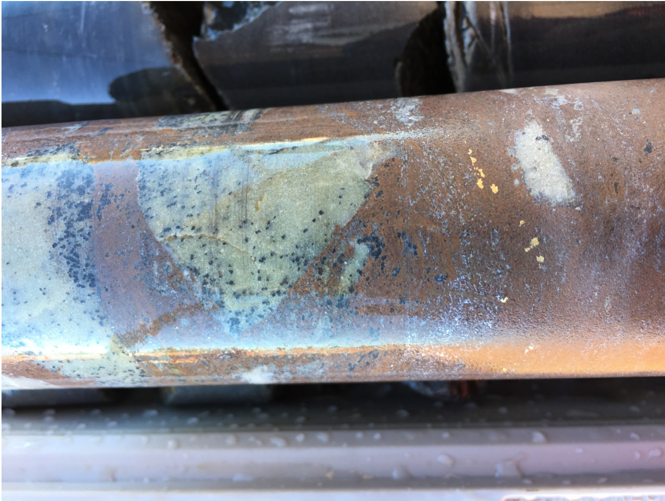
Siliceous breccia with low-iron sphalerite and visible gold. Black spots are intimated intergrowths of tremolite and galena. Hole HRUD525, Far West Lode.
