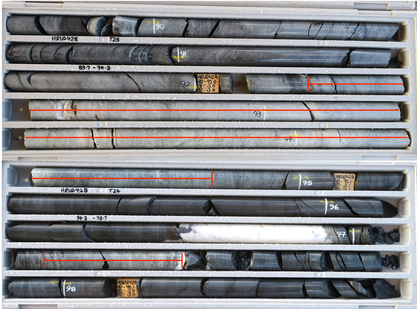
Broad, unmineralised tremolite-zoisite-anorthite skarn intercept from the footwall of North Pod. Zoisite ( var thulite ) is light pink in this zone indicating elevated manganese.
