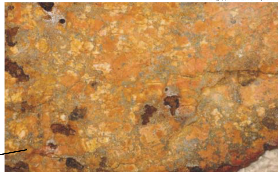
Gold-bearing greisenised granite from Seven Hills
