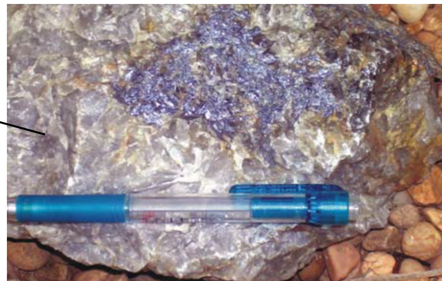
Moly in Qtz pipe from Kingsgate Mo-Bi prospect
